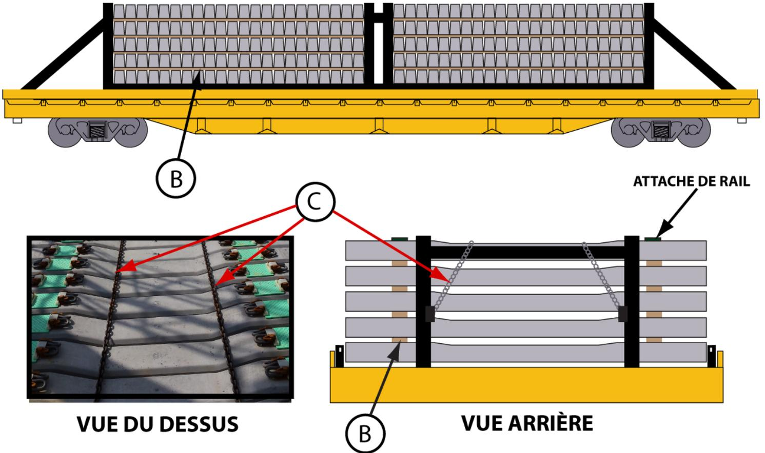
TRAVERSES, BÉTON – WAGON POUR TRAVERSES DE BÉTON
