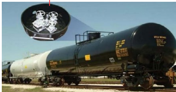
Valving inside the \frac{3}{4} " protective housing
