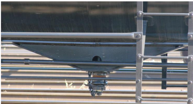
Bottom outlet valve on tank car, skid protection – external view
