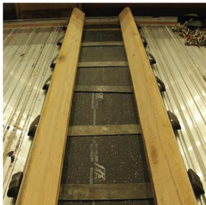
COIL BEDDING (INSIDE VIEW)
