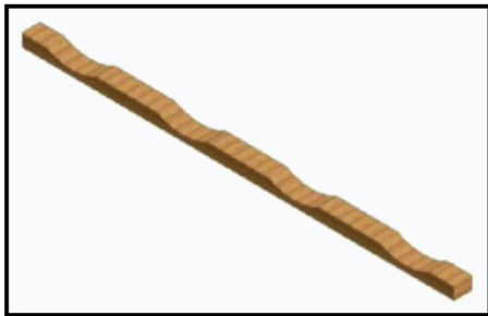
SPRUCE BEARING PIECE FULL 4 in. X 6 in. CONTOURED TO FIT PIPE SKETCH 5
