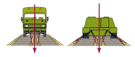
♦ When loading military tank on a rail equipped car (i.e.: HTTX) or general-purpose flat car, only **ONE** tank must be loaded and centrally located on the rail car. No other vehicles can be loaded to use the vacant space at front and rear of the tank.
