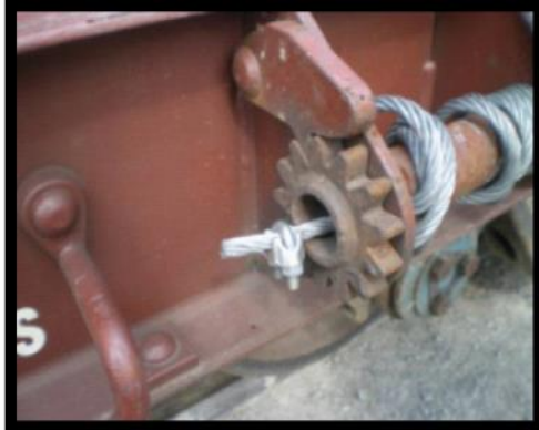
Improperly fitted clamp on ratchet barrel
