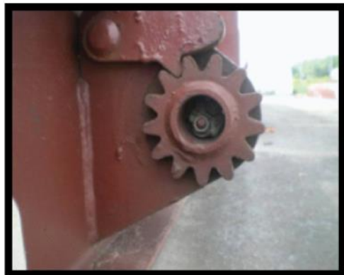
Properly fitted bolted clamp on ratchet barrel
