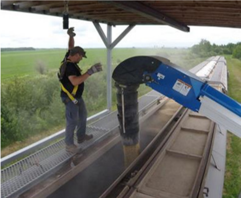
Figure 9. Shipper’s loading system to transfer agricultural product from truck to covered hopper railcar on Ontario’s Northland’s spur line
