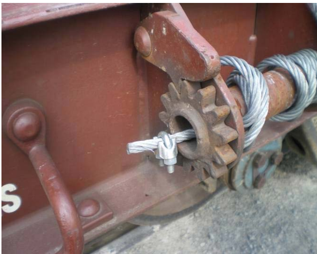
Improperly fitted bolted clamp on ratchet barrel
