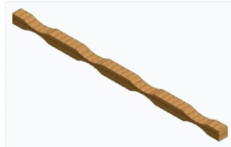
SPRUCE SEPARATOR FULL 2 in. X 6 in. CONTOURED TO FIT PIPE
