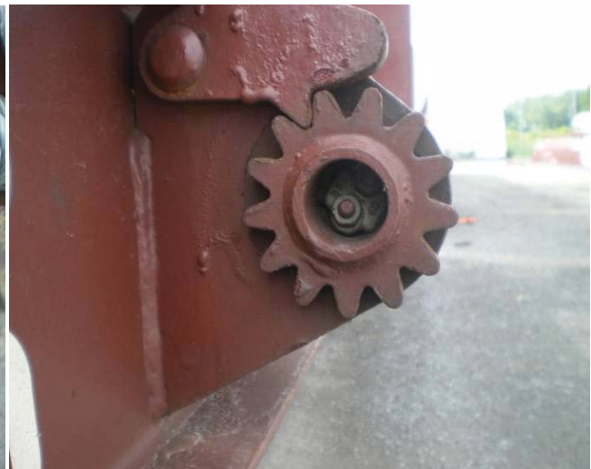
Properly fitted bolted clamp on ratchet barrel
