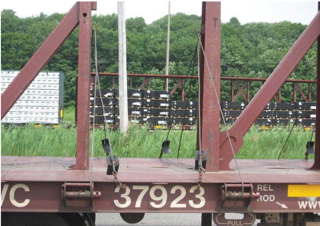
Properly secured cable for empty movement of railcar
