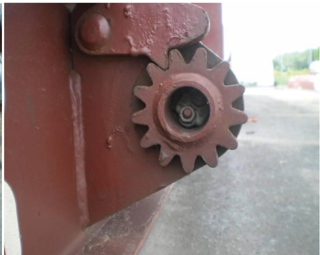
Properly fitted bolted clamp on ratchet barrel
