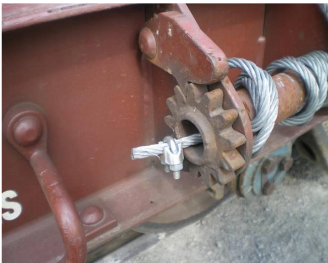
Improperly fitted bolted clamp on ratchet barrel
