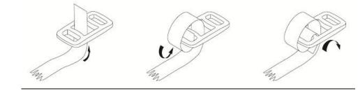
**Step 1.** Feed strapping up through center gap
