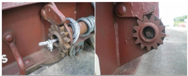
Improperly fitted bolted clamp on ratchet barrel
