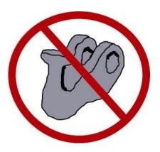
**NOTE:** To properly secure a tank on a rail flat car, use the 21-ton capacity bolt shackle (NSN 4030-21-256-2423) to secure the tank. No other type of shackles (i.e.: towing hook, as in above graphic) is allowed to secure the tank.
