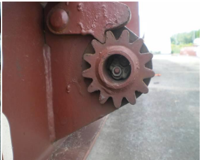
Properly fitted bolted clamp on ratchet barrel
