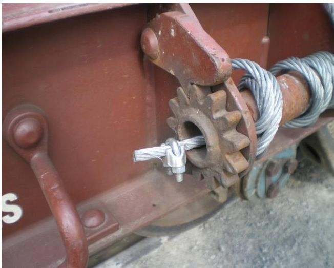
Improperly fitted bolted clamp on ratchet barrel
