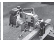
High Speed Rail Drill - Gas
