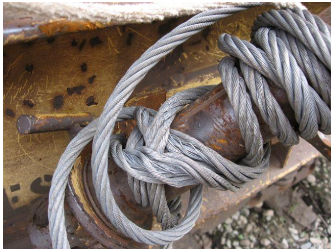
c) Flattened cross-section (crush cable)/ Kinks greater than 60°
