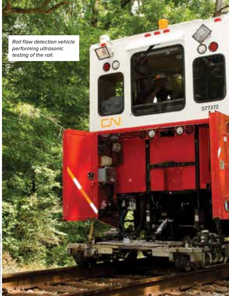
Rail flaw detection vehicle performing ultrasonic testing of the rail.
