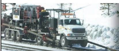
Rail Unloading Machine (R.U.M.)
