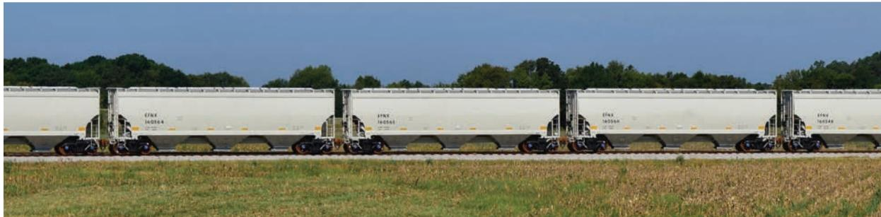
As part of its expanding product portfolio, FreightCar America has been meeting North America fleet demands for 5,200 cubic foot covered hopper cars for grain service. These cars feature patented high strength cold-rolled center sills that, along with other engineering design elements, help reduce tare weight and enhance payload capability. These innovative cars are part of a growing, diverse line of highly productive railcar designs from FreightCar America.
