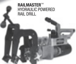
**Move fast.** Time is essential when making changeouts. Trak-Star® Rail Drills and Saws are ergonomically designed for easy one-person operation. Choose from gas or hydraulic power. Light weight tools and unique 10-point rail clamps make moving from cut to cut fast.
