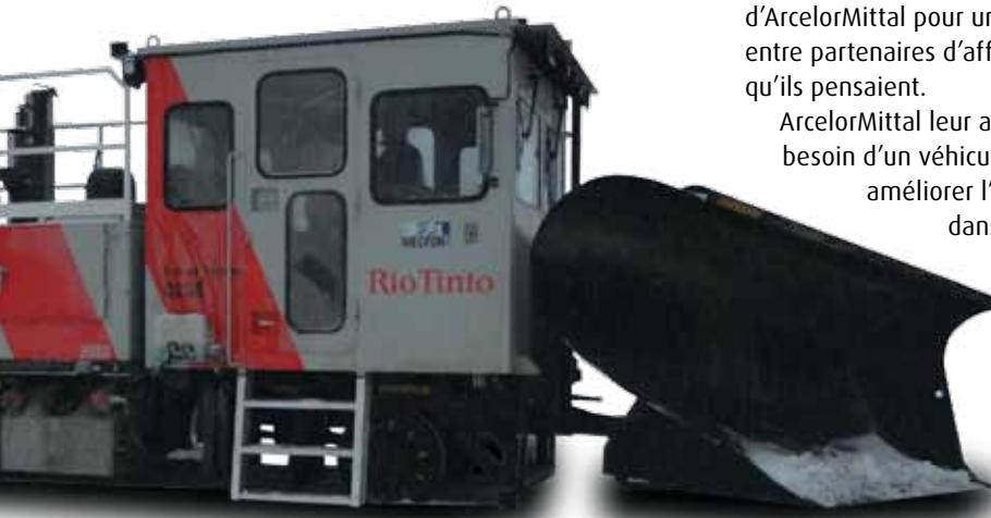
ArcelorMittal recognized that its employees responsible for repairing the company's rails were occasionally exposed to dangerous working conditions in isolated regions. In an effort to maintain productivity while improving safety, the UTV was designed to provide railway transportation to workers as well as carry the tools needed for track maintenance over long distances.
